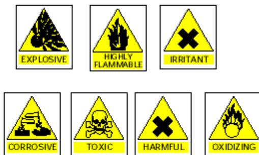
**Fig. 6.3 Seven main symbols for hazardous substances**
