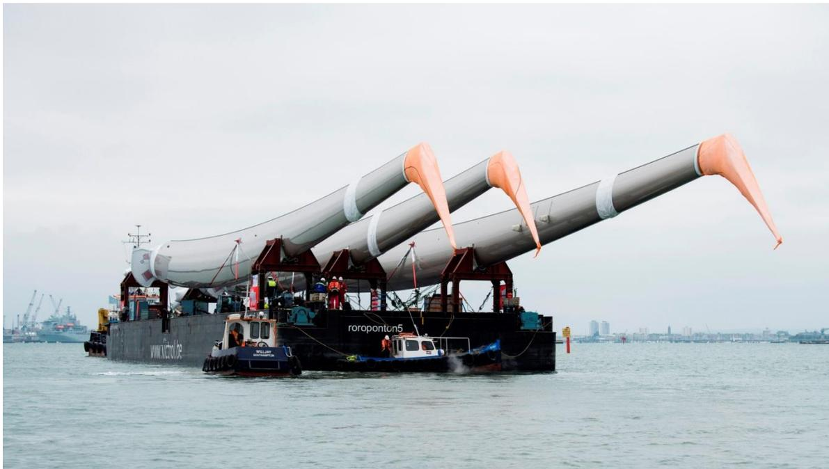
Composites specialists, Magma Structures have delivered three of the world's tallest carbon composite free-standing masts. The rigs are designed to withstand bending loads of more than 40Mn; more than twice the load on a Boeing Dreamliner wing. The masts were ordered by a German shipyard and are destined for a sailing superyacht.
