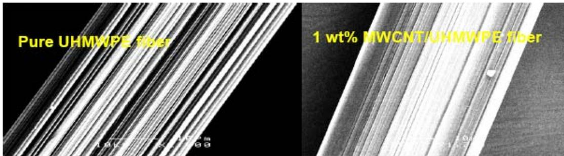
**Figure 6** UHMWPE and MWCNT/UHMWPE composite (Lee 2005).
