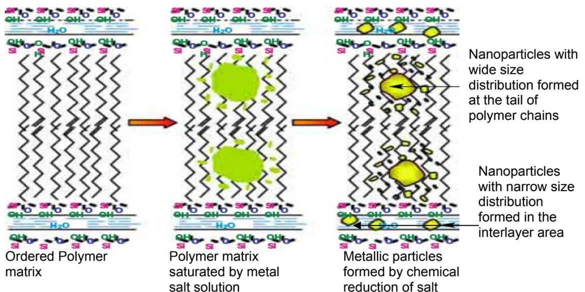
**Figure 4** Formation of nanoparticles in polymer matrices (Global Watch 2005).
