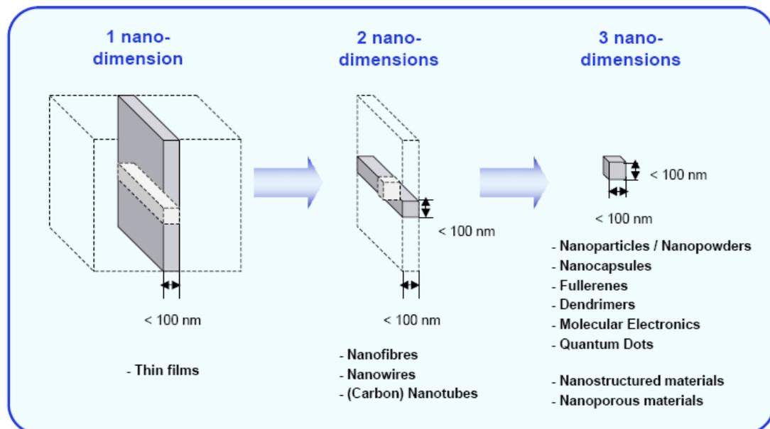
**Figure 1** The classification of nanomaterials according to their dimensionality (NRM Report).
