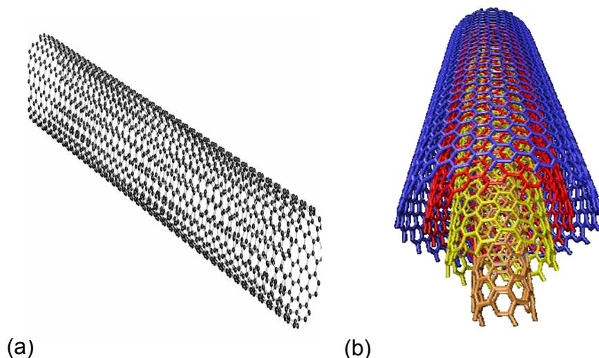
**Figure 2** Schematic of carbon nanotubes (The Royal Society Report):
