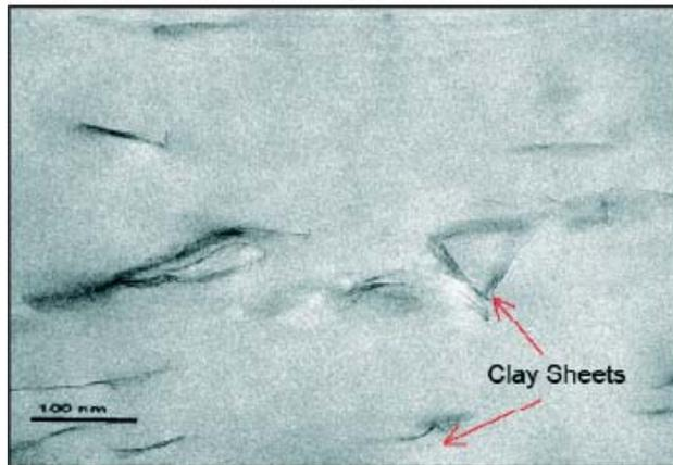
**Figure 5** Transmission electron microscopy (TEM) of a polymer-layered silicate NC prepared in a twin screw extruder (Gacitua et al, 2005).
