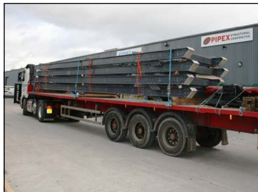
(Shoring packed onto 1 lorry for delivery)
