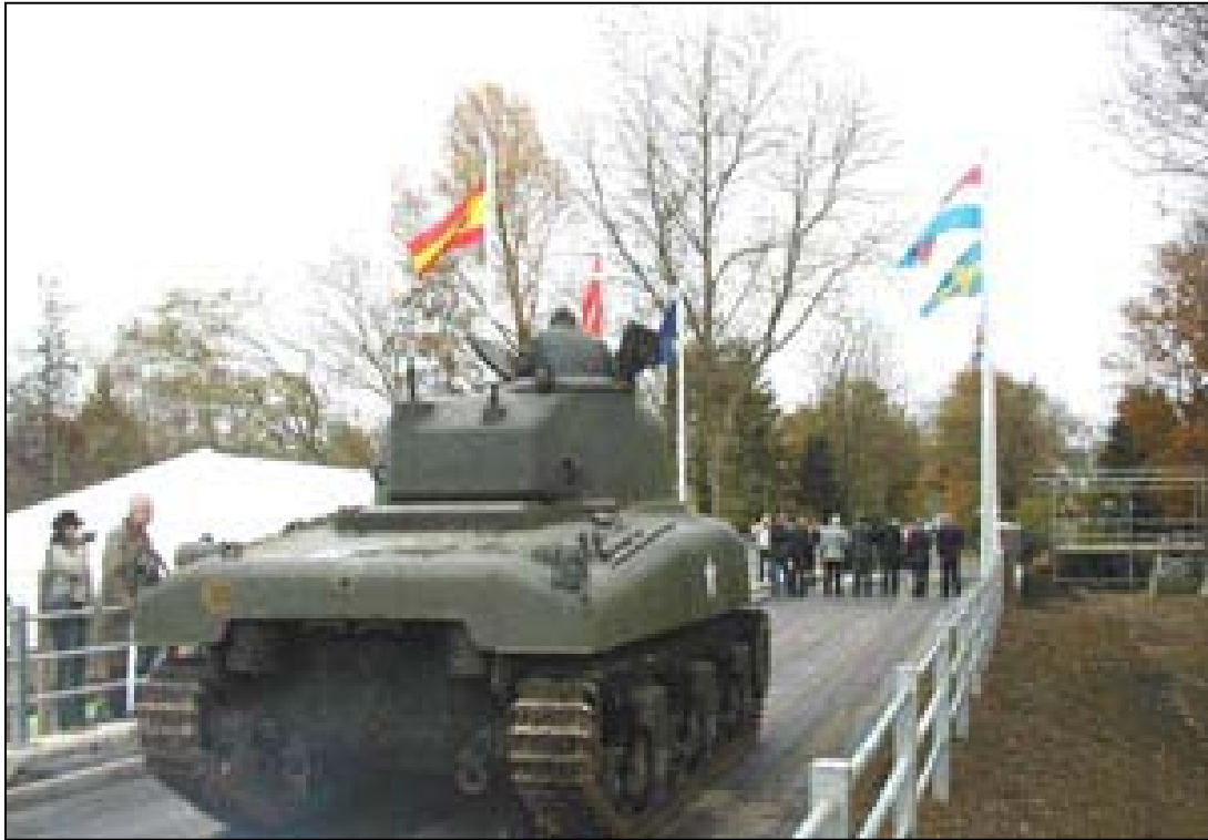
Figure 2. Military tank used for on-site testing of Mouchel designed bridge (Courtesy of Mouchel Parkman )
