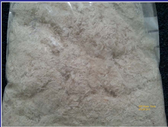
GRP waste: offcuts, shredded and ground material Photos courtesy of Filon Products Ltd
