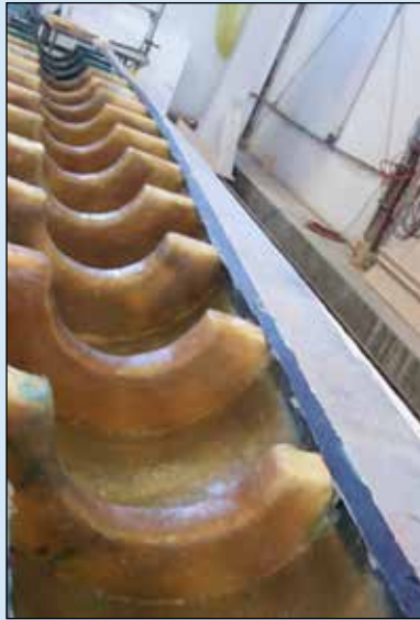
FIGURE J.9-2: Stiffening ribs placed within a curved FRP structural member
