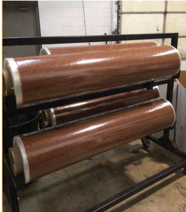
Figure 11: Cashew nut shell liquid based Flax Coral Prepreg, produced by CTS, Ohio. Photo courtesy of Elmira Ltd, UK.
