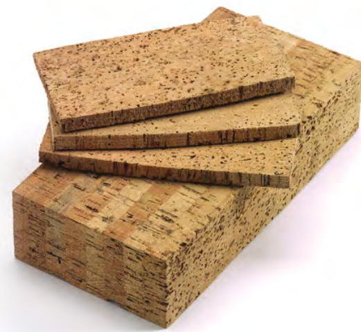
Figure 12: Granulated cork formed into a sheet, courtesy of Amorim Cork Composites.
