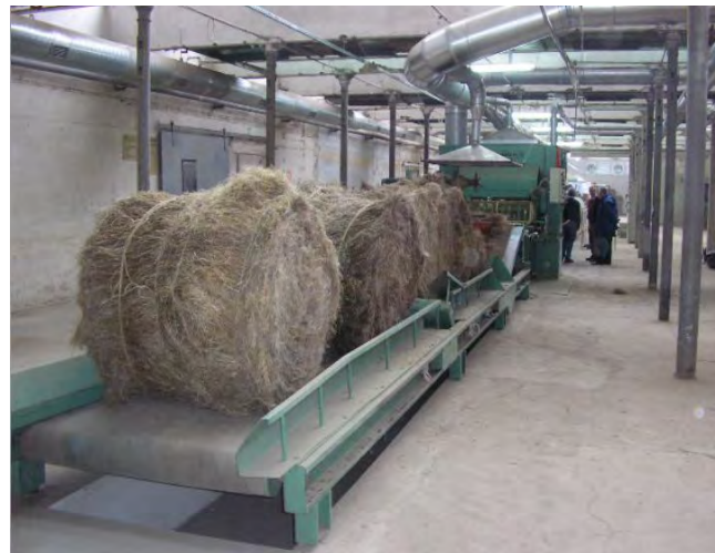
Figure 4: Bale opening at the start of a flax processing line (photo used with kind permission of Mr Marian Planik, WFB Baird Poland Sp. z o.o.).
