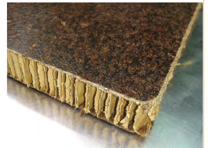
Figure 16: Flax / bioresin / paper honeycomb sandwich by EcoTechnilin. Photo:Stella Job, Materials KTN
