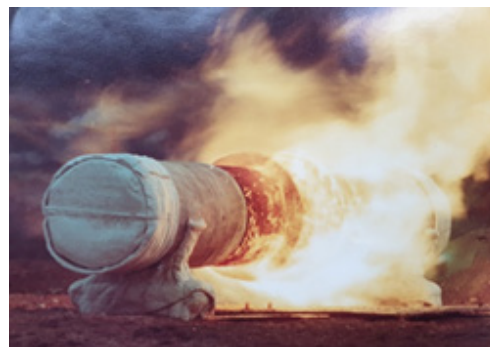
Photo courtesy Tom Royle: Jet fire test on riser protection system at Spadeadam
