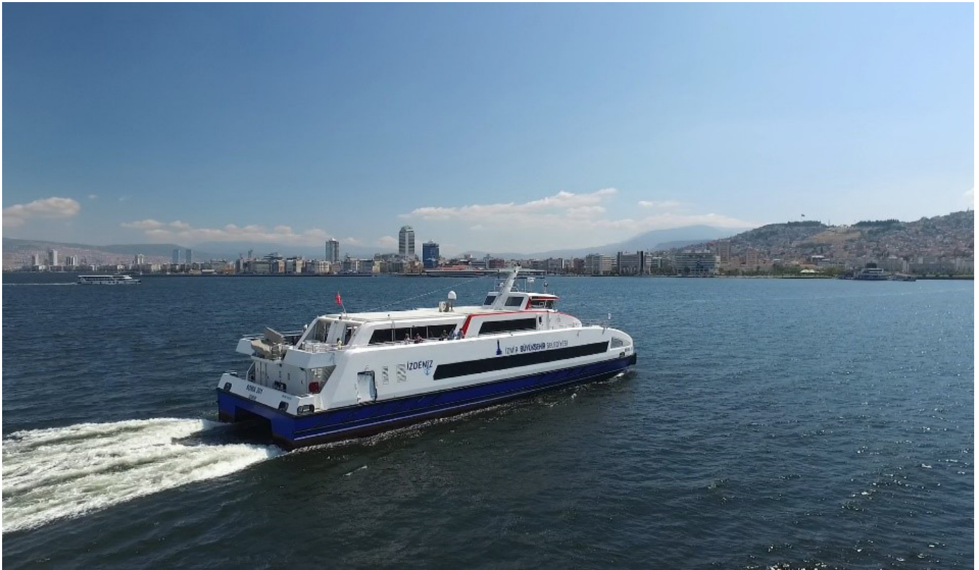
One of 15 carbon fibre 39m, 32 knots, catamaran ferries. Photo courtesy of Sigmatex on behalf of Özata Shipyard, Turkey.
