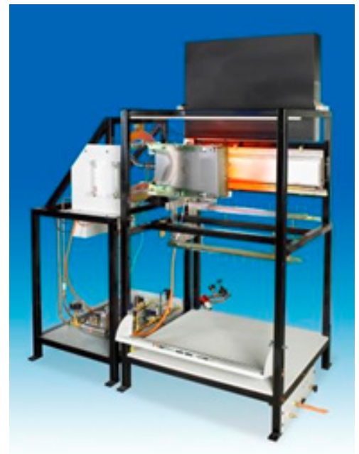
Photo courtesy Fire Testing Technology: ISO 5658-2; IMO Resolution A.653(16); ASTM E1317; ASTM E1321 Spread of Flame Test Rig
