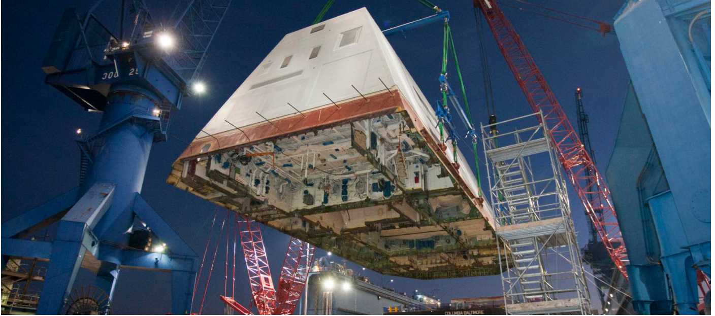
900t composite deckhouse of USS Zumwalt being lifted into position. Photo: US Navy
