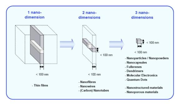
Figure 1 The classification of nanomaterials according to their dimensionality (NRM Report).
