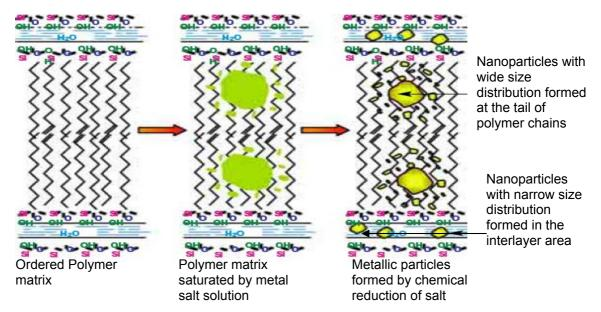
Figure 4 Formation of nanoparticles in polymer matrices (Global Watch 2005).
