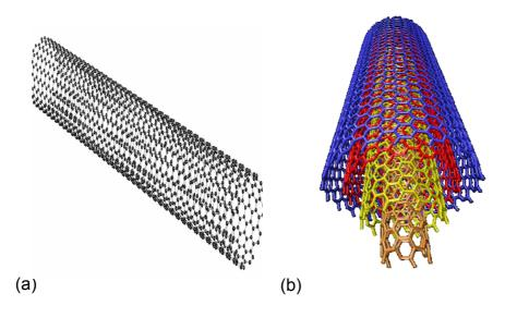
Figure 2 Schematic of carbon nanotubes (The Royal Society Report):
