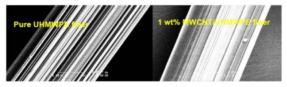
Figure 6 UHMWPE and MWCNT/UHMWPE composite (Lee 2005).
