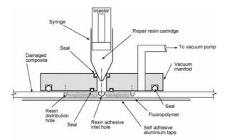
Figure 6 - Resin Infusion or Injection Repair
