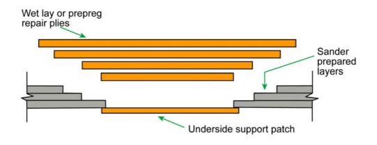
Figure 3a: Stepped Scarf Repair
