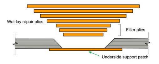
Figure 2: Laminated Patch Repair
