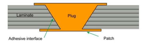
Figure 5 - Adhesive Bonded Plug Repair
