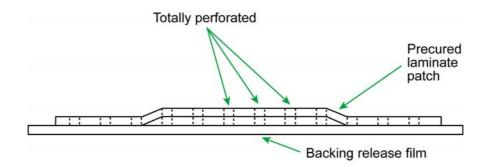
Figure 4 - Adhesive Bonded Doubler
