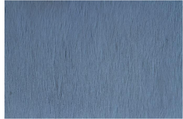
Aligned mats made with 50% and 100% rGF
