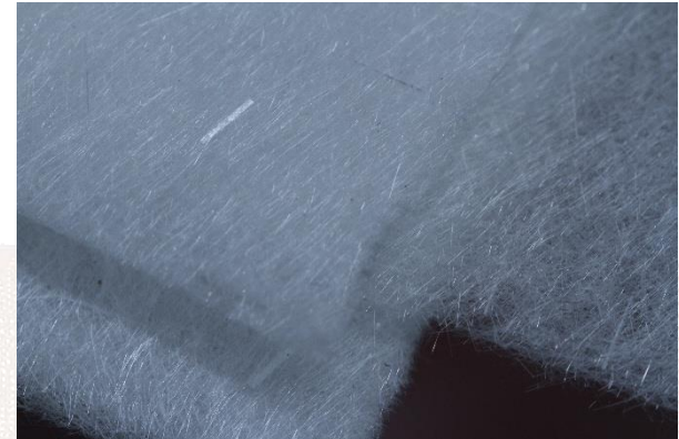
Non-Aligned mat made with 50% and 100% rGF
