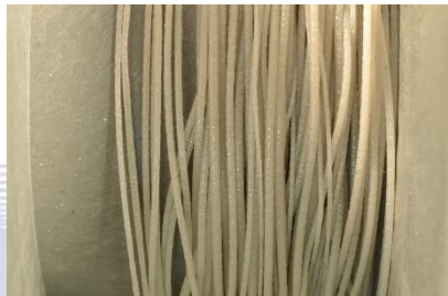
3D printing filament (100% rGF)
