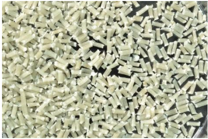
Pelletised rGF filled PP composites for injection moulding process (100% rGF)
