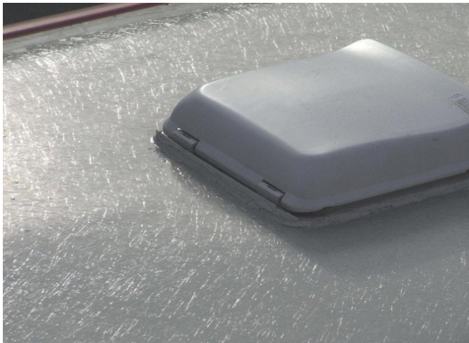
Roofing sheet incorporating recovered glass fibres, used in a campervan roof. Photo Stella Job.
