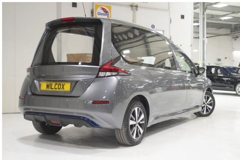
Wilcox hearse with recycled carbon fibre bodyside. Photo courtesy of Prodrive Composites
