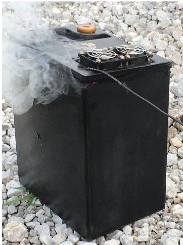
Figure 5.2: PS200 glass fibre PFA battery box undergoing fire test. Photo courtesy of SHD Composite Materials Ltd
