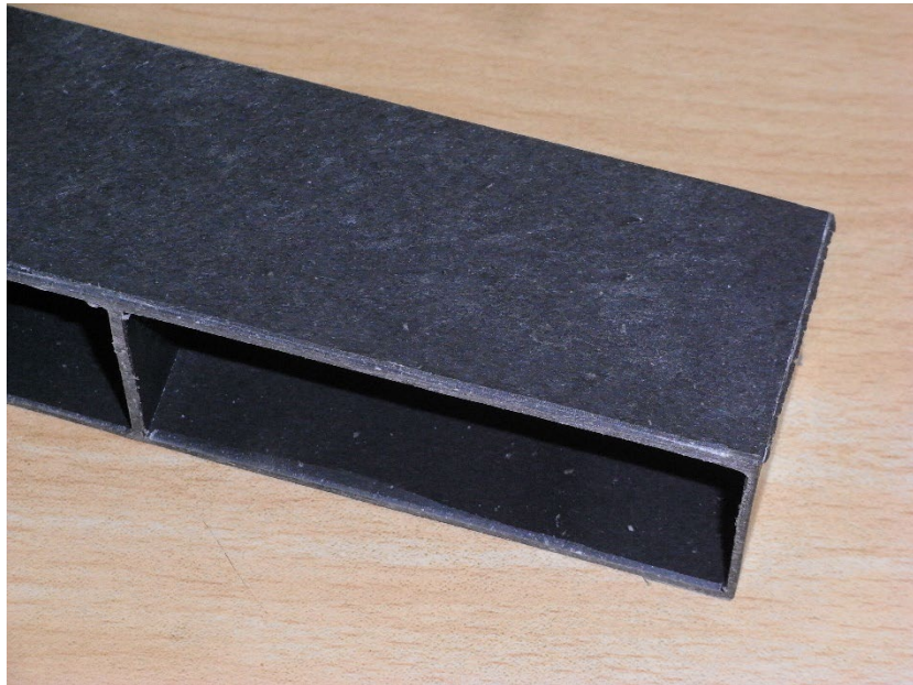
Injection moulded part using glass fibres recovered from GRP regrind compounded with polypropylene. Photo: Stella Job
