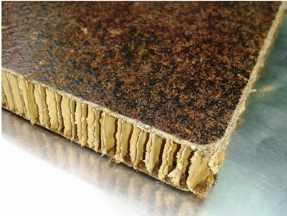
Ecotechnilin Fibricard, flax / PFA with paper honeycomb core, as used in Jaguar F-type boot load floor, 2013. Photo Stella Job
