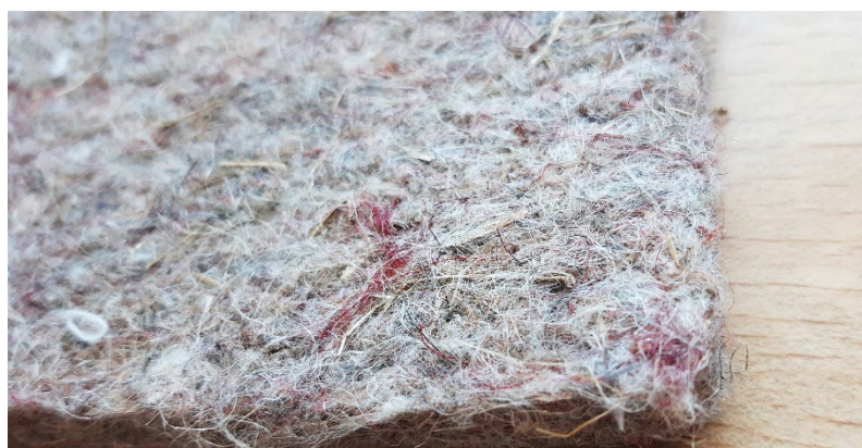
Ecotechnilin flax/PP 1600 g/m 2 felt, used in Opel Insignia boot trim, using PP fibre waste from carpet production. Photo Stella Job
