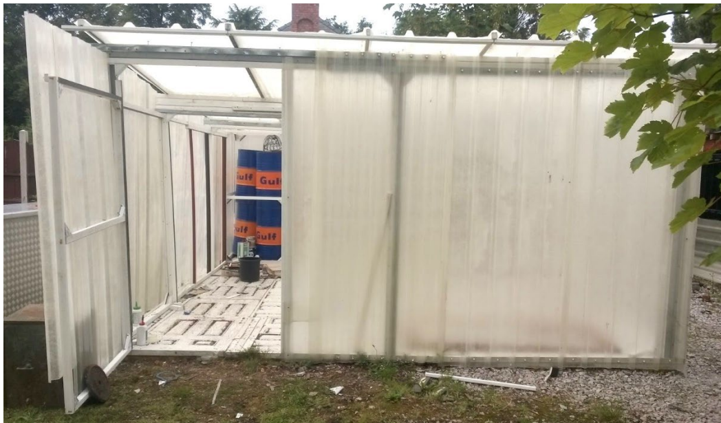
Figure 4.2: Greenhouse made from GFRP sheets & composite door edge offcuts. Photo courtesy of Paul Ridley, Cabinz
