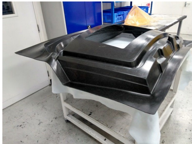
Recycled carbon fibre tooling for hearse tailgate structure. Photo courtesy of Prodrive Composites
