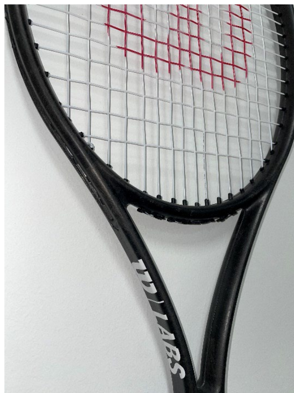
Carbon fibre tennis racquet incorporating 50% reclaimed carbon fibre, aligned using Lineat technology. Photo courtesy of Lineat
