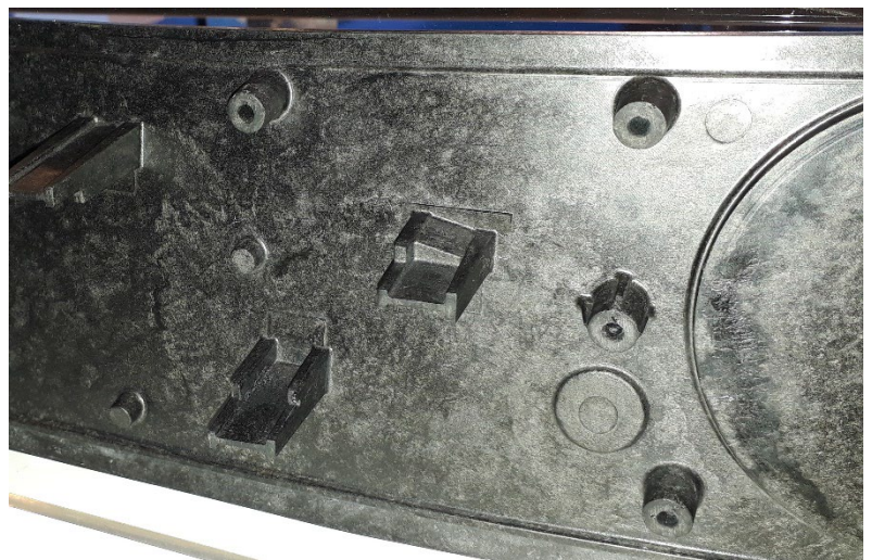
Complex moulded part using moulding compound produced from uncured prepreg waste. Photo: Stella Job
